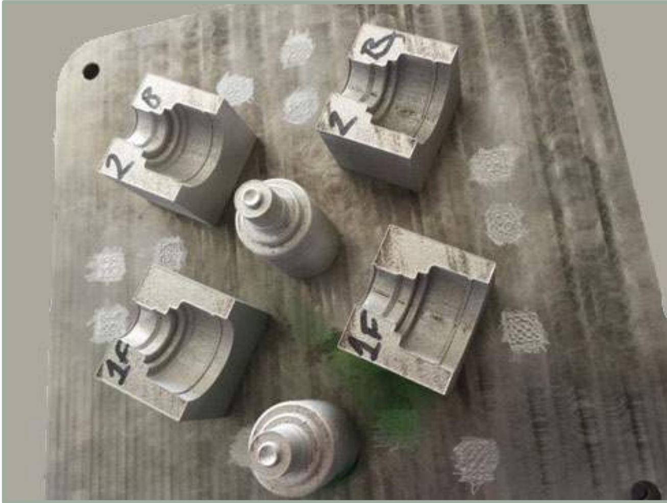
Figure 12 - Parts on the build platform
