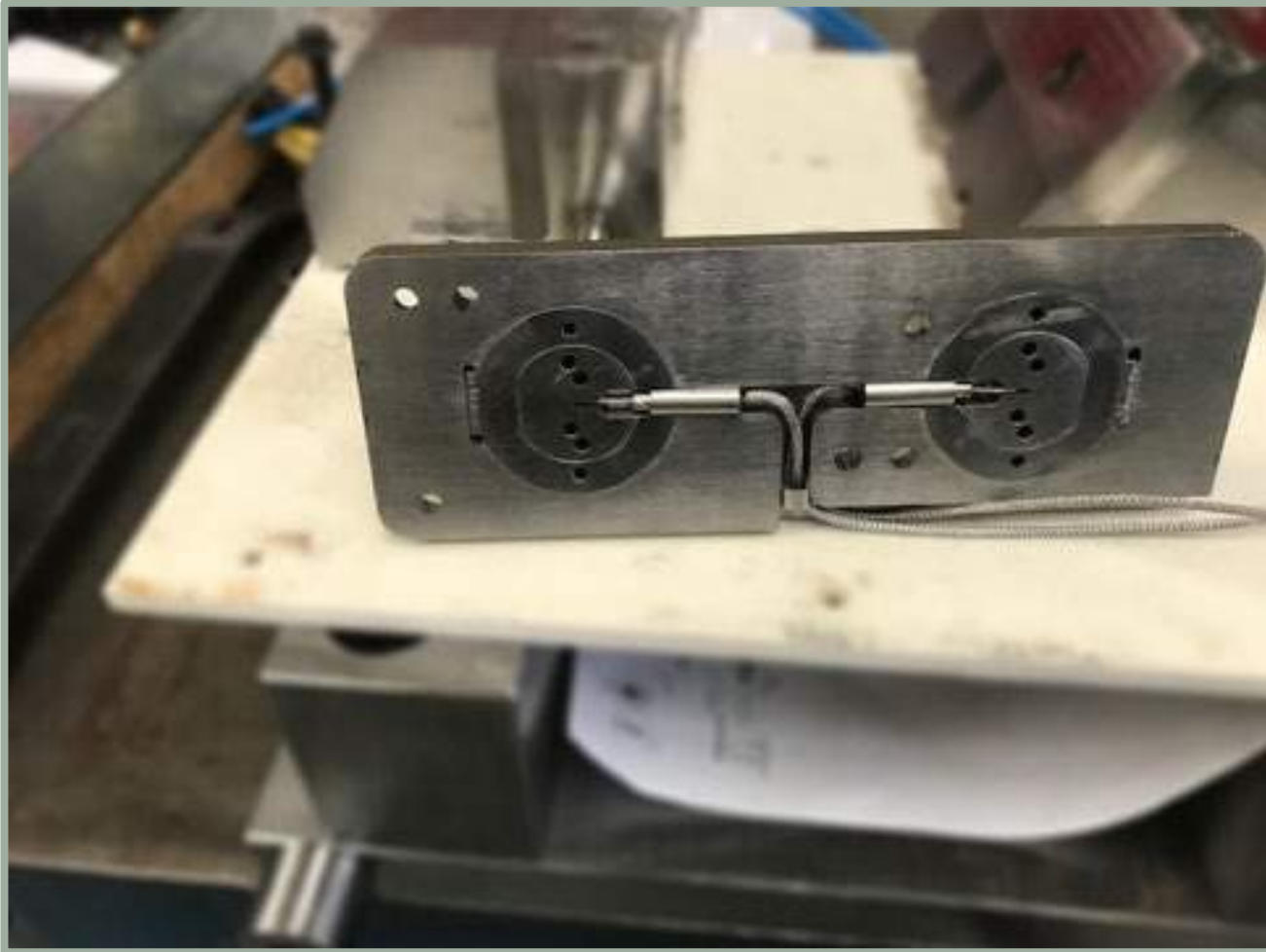
Figure 9 - Thermocouple fitted to core
